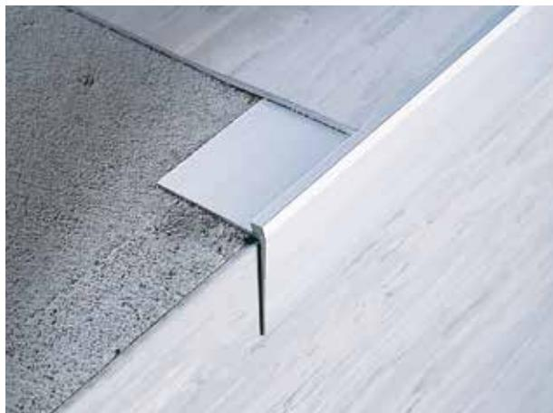
STAIRTEC SC stair nosing profile is designed for thin, resilient flooring. Simply lay the flooring on the step riser, install the profile covering the riser edge and then apply the tread flooring flush in the indented lip of the profile. STAIRTEC SC profile protects the tread edge and hides riser imperfections.
